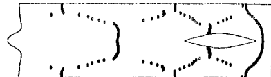
b) Subsonic. Bow shock has detached. Shocks behind the body are from bow shock reflections with the cylindrical boundary.
